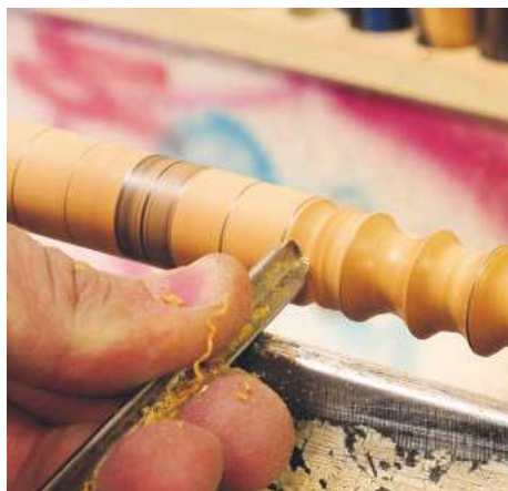
▲ Pic.32 Cut a series of covers along the length, working from the tailstock end towards the headstock. Not only do they look decorative but they will also stop the jewellery falling off
